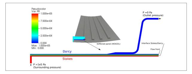
Figure 1: Pressure fields in macroscopic scale simulation of resin infusion manufacturing process for a slice of stiffened panel.
