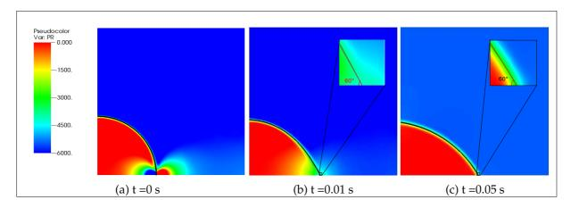
Figure 2: Discontinuous pressure fields in the simulation of bubble interface evolution with a contact angle of 60°.
